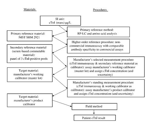
**Figure 2** Suggested approach for the standardization of cardiac troponin I (cTnl) measurements through traceability implementation to the reference measurement system. RP-LC, reversed-phase liquid chromatography.
