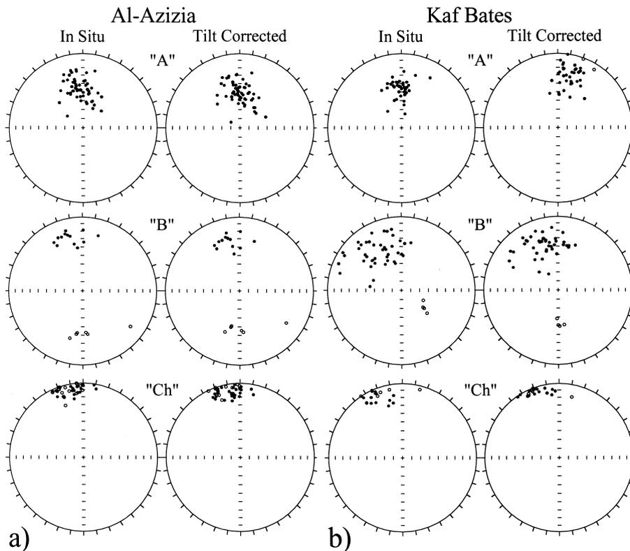
Fig. 5. Equal area projections before (in situ) and after bedding tilt correction of the 'A', 'B' and characteristic 'Ch' component directions from (a) the Al Azizia and (b) the Kaf Bates section of the Al Azizia Formation.
