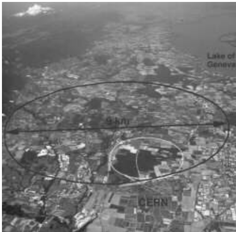
Circular configuration of the LEP 28 km (17-mile) underground tunnel near Geneva, Switzerland.
